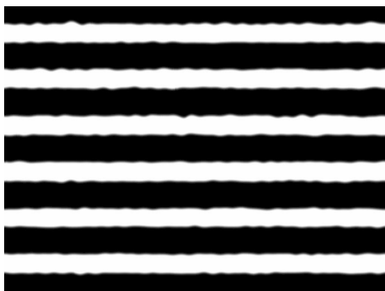
Fig. 12. Computed aerial image with monopole \sigma = 0.05 illumination and 100-nm wafer defocus.
