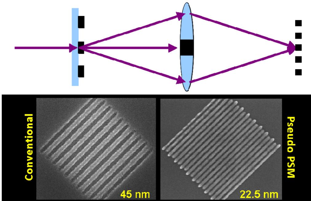
**Fig. 4.** Schematic of the pseudo-PSM process along with exposures of 45-nm lines and spaces using both conventional illumination and the Pseudo-PSM method which results in twice as many 22.5-nm lines and spaces.
