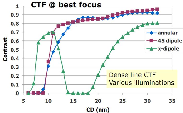
Fig. 12. Modeled performance of 0.5-NA system in imaging equal lines and spaces under three different illumination conditions.
