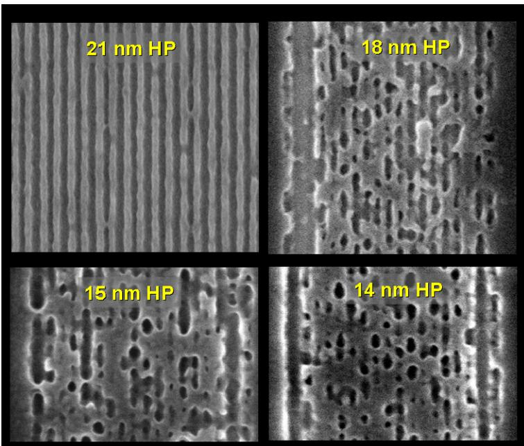
**Fig. 6.** Pseudo-PSM mode printing in BBR-08b demonstrating that we are not mask limited in terms of resolution.
