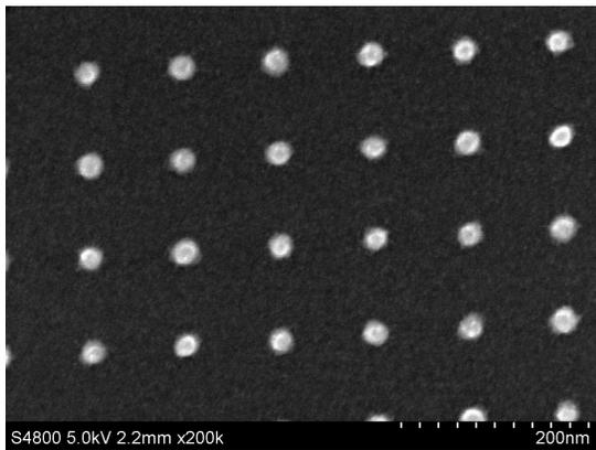
**Fig. 8.** 22-nm posts printed in the Inpria material using conventional annular illumination.
