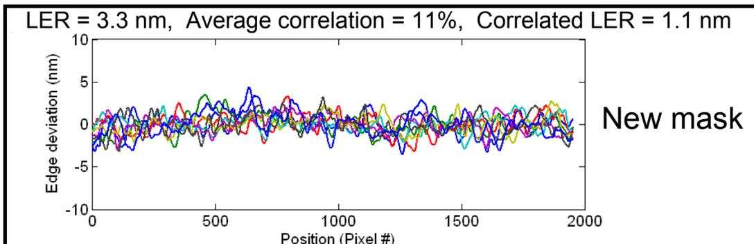
**Fig. 10.** Correlated LER measurement on new mask with  $\sigma = 0.5$  and 100-nm defocus.
