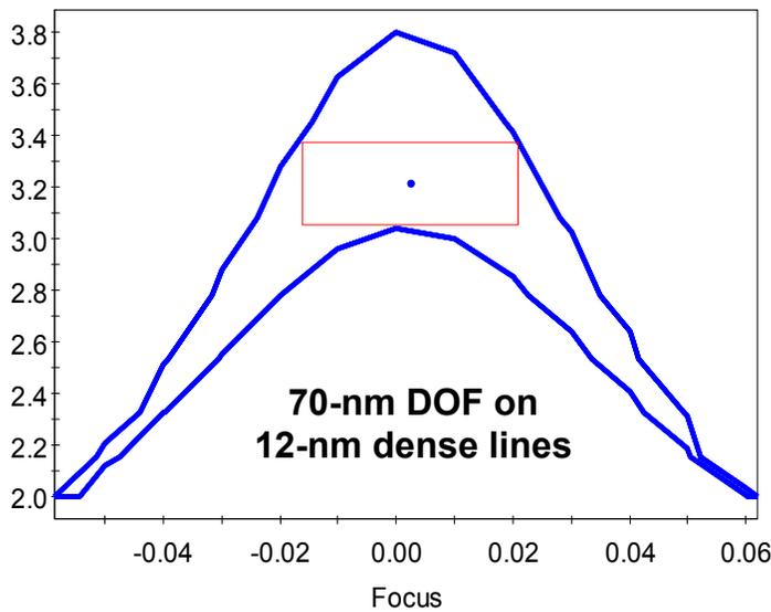
Fig. 13. Modeled process window performance of 0.5-NA system in imaging 12 nm equal lines and spaces using conventional annular illumination.
