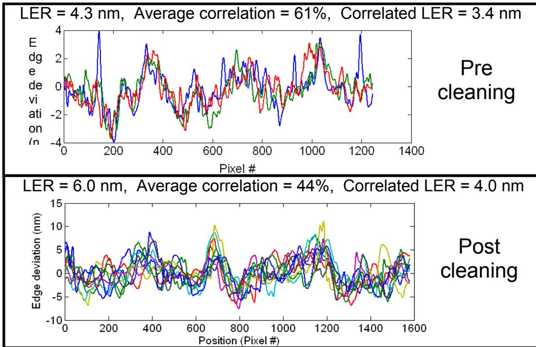
**Fig. 9.** Direct comparison of the correlated LER measurement at the exact same area on the mask increase is 0.6 nm and the uncorrelated LER increase is 1 nm.
