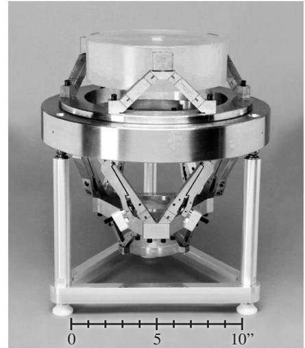
Figure 1: Photo of the MET optical system resting on a stand. Photo courtesy of John Taylor, LLNL.
