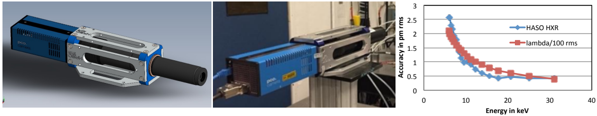
Figure 11. LEFT, rendering of the optimized HXR wavefront sensor at Imagine Optic SA . CENTER, The WFS installed at the APS 7-ID beamline. RIGHT, Calculated accuracy of the wavefront sensor, compared with a \lambda/100 value.
