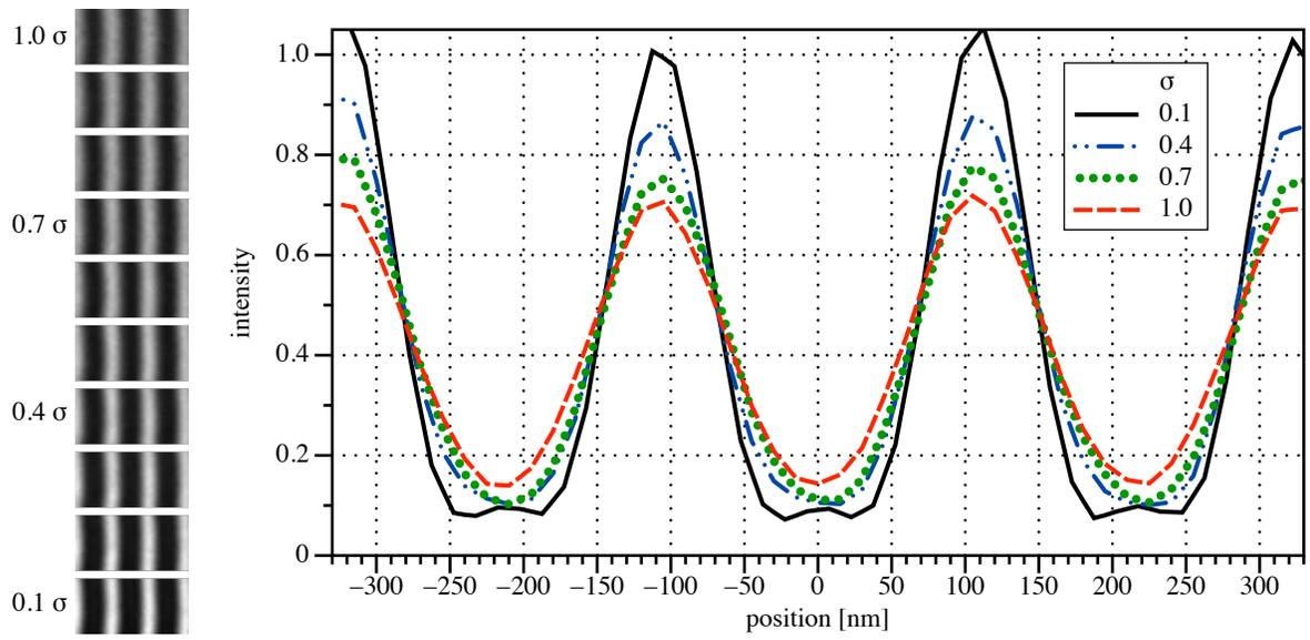
Figure 4. Line intensity profiles extracted from the circle grating pattern in the 3 o'clock position. The profiles share a common intensity normalization, showing that the coherent light ( $\sigma = 0.1$ ) has the globally highest peaks. At this line size and NA, higher  $\sigma$  values are associated with reduced contrast, and lower image intensity slope. (Color online.)
