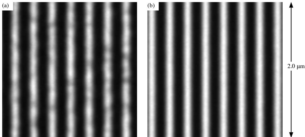
Figure 8. Two similar regions of an experimental mask that has been prepared to contain varying levels of substrate roughness. The measured LWR  $3\sigma$  values for 2- $\mu\text{m}$  line segments were (a) 16.6-nm and (b) 3.2-nm.
