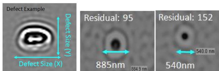
Figure 2. A defect image obtained at 193nm is shown on the left, with size in x and y superimposed. The smaller defect images on the right illustrate that size and residual do not always correlate: the defect that is larger has a smaller residual signal in this case.
