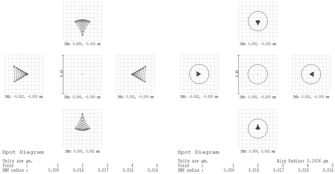
Figure 5. In-focus spot diagram of the central field point and field points 2  $\mu\text{m}$  off center at the mask side for the off-axis configuration: (left) regular spot diagram; (right) spot diagram and Airy disk.
