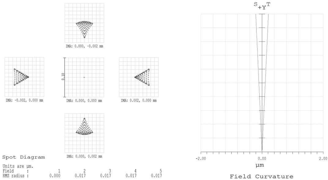
Figure 6. In-focus spot diagram of the central field point and field points 2  $\mu\text{m}$  off center at the mask side for the on-axis configuration at 3-mm working distance and a magnification of 333.
