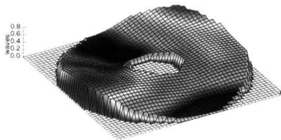
Fig. 13 Wavefront variations measured for an annular zone plate lens at 13 nm wavelength using an earlier version of the PDI. The dominant aberration is 0.26 waves of astigmatism, some of which may be associated with an overly large reference pinhole used at that time (from Ref. 33).
